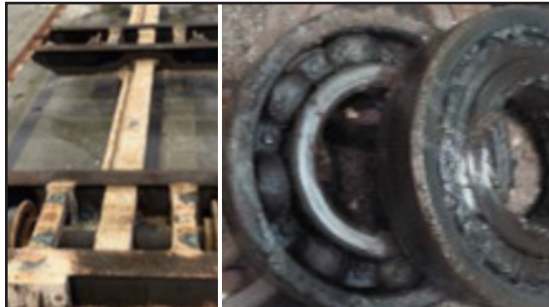
Failed bearings on autoclave transport rigs.
